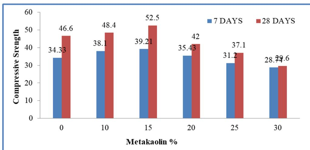
**Figure 3.1. Graph showing Compression Strength at various proportions of Metakaolin**
