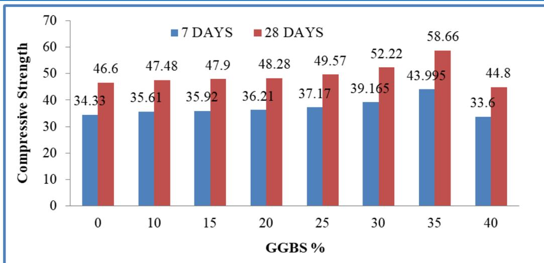
Figure 3.2. Graph showing Compression Strength at various proportions of GGBS %
