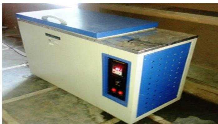
Figure 2.4. Accelerated Curing Tank
